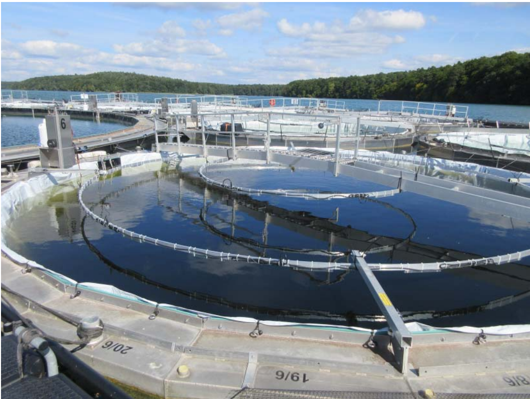
Figure 2. One of the LakeLab's nine-meter-diameter enclosures. Note the concentric lighting "rings" above the mesocosm. Photograph by author.
