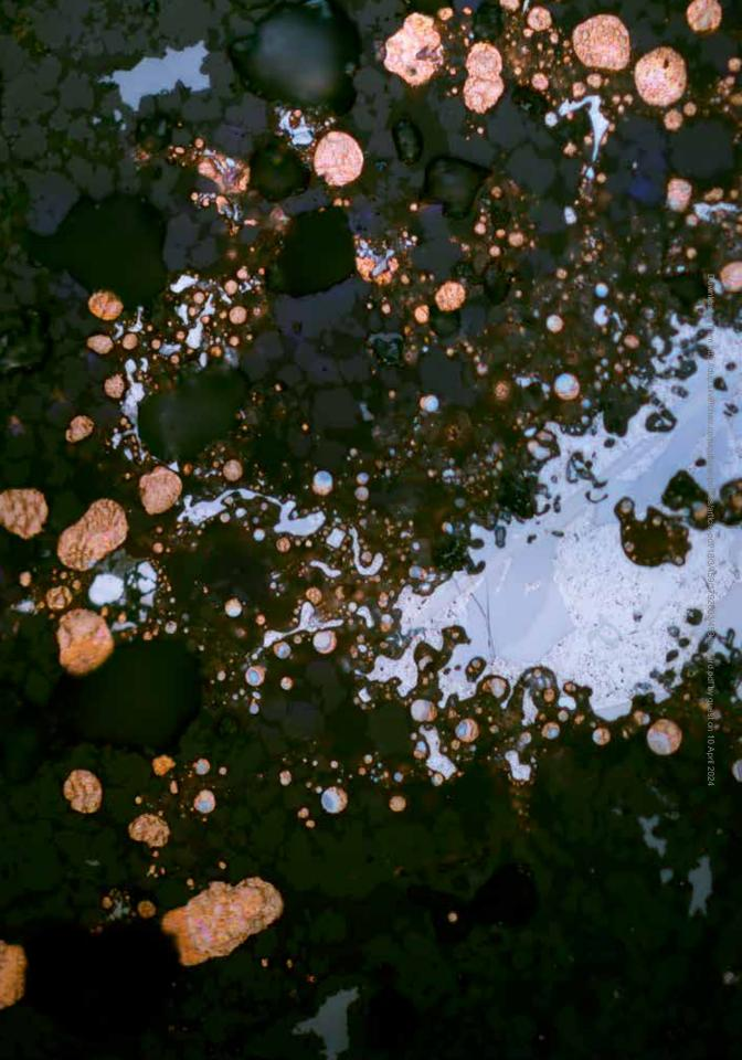
crucible and binding the unfolding melt to it. At 1300°C tinges of rich cobalt emerge from the battery, and by 1400°C this blue has spattered the crucible's surface as microstalagmites bubble up out of the glistening gray mass. At 1500°C any definition between individual components vanishes as the last melting points are surpassed, collapsing into a gun-metal agglomeration.
